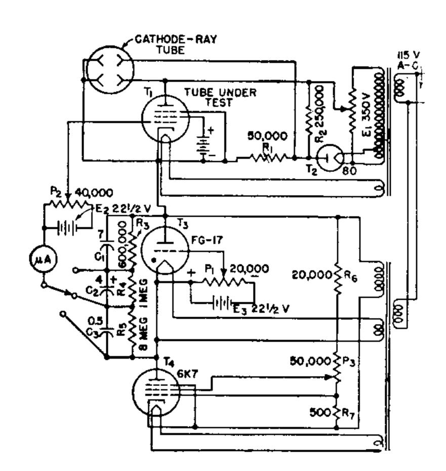
circuit constants. The microammeter in the grid circuit of the tube under test facilitates the adjustment of  $P_2$ .
